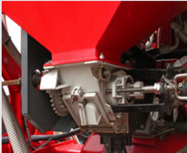
Modern, universal FX metering unit guarantees a repeatable metering dose ranging from 1.8 to 400 kg/ha. The metering unit is suitable for fine and coarse grains, with no need to replace the metering rollers. Easy adjustment and accurate setting ensure seamless seed dosing. The metering unit is featured with a quick system removing seed residues.
