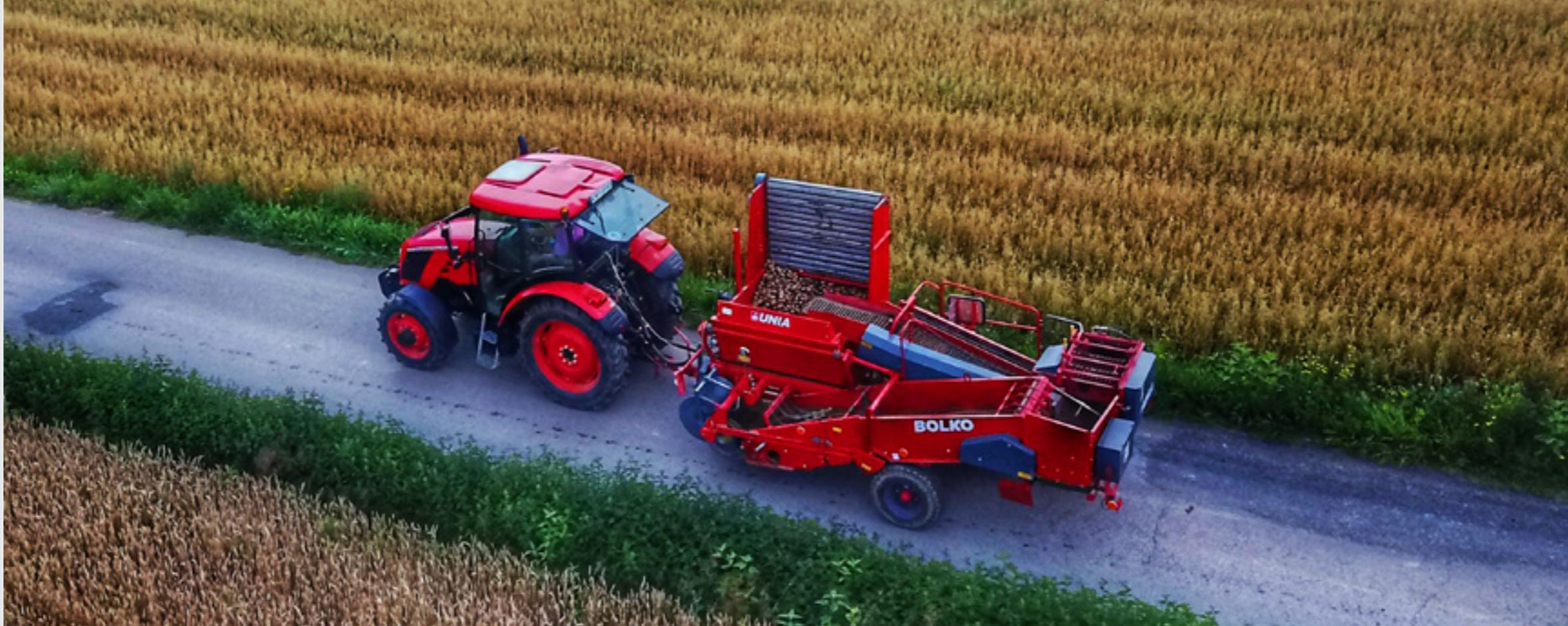
The harvester drawbar is featured with a hydraulic cylinder which enables shifting the harvester to a working position and facilitates maneuvering during transport or potato unloading.
