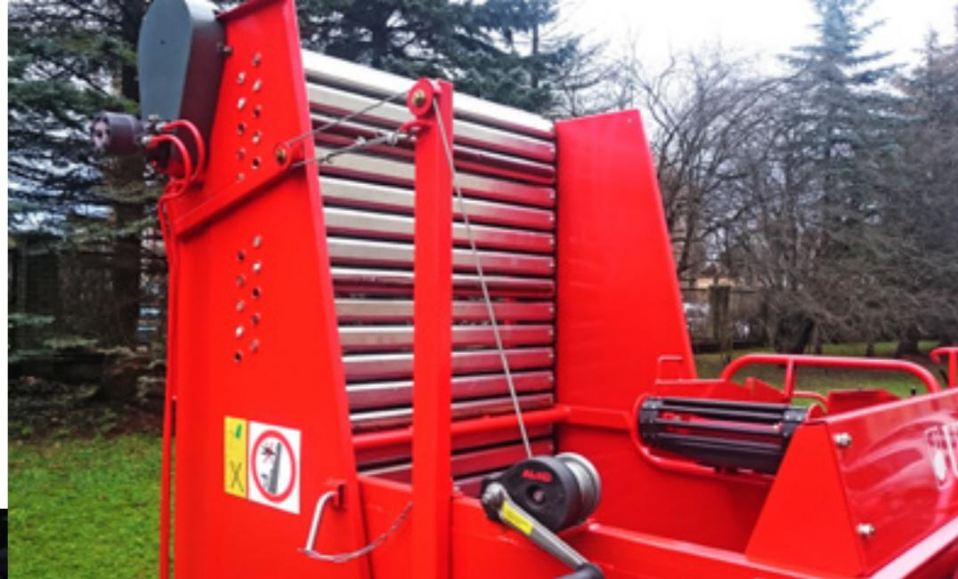
BOLKO is equipped with a potato hopper with the maximum load capacity of 1250 kg. The hopper is unfolded and folded mechanically with a special crank.
