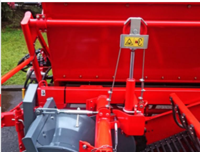
The operation of the ground-following roller is adjusted with a tensioning screw, while the whole digger is hydraulically lifted and lowered.
