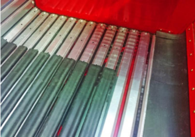
To avoid potato damage, the floor conveyor is equipped with ca. 80 cm long rubber guards.
