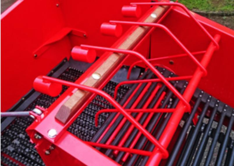
The gap between the intake roller and the scraping slat should be as small as possible, whereby the roller should not rub against the slat. The gap is adjusted by moving the slat aside or towards the roller, after loosening the screws. If stems wind around the intake roller (wide gap between the roller and the slat), they can be removed by being cut with the hook which is the harvester equipment.
